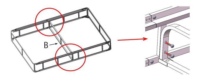
STEP 3: Assemble the two middle support rail bars, two ends with M6\*25 screw and gasket, the middle with M6\*50 screw ,nut and gasket (not including Twin).
